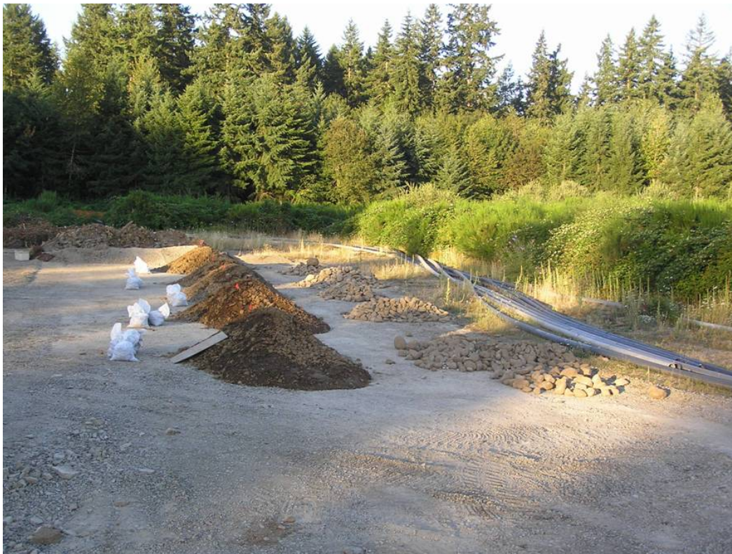
Figure 2. Plus and minus 127-mm (5-inch) sample fractions (minus 127 mm on the left and plus 127 mm on the right).
